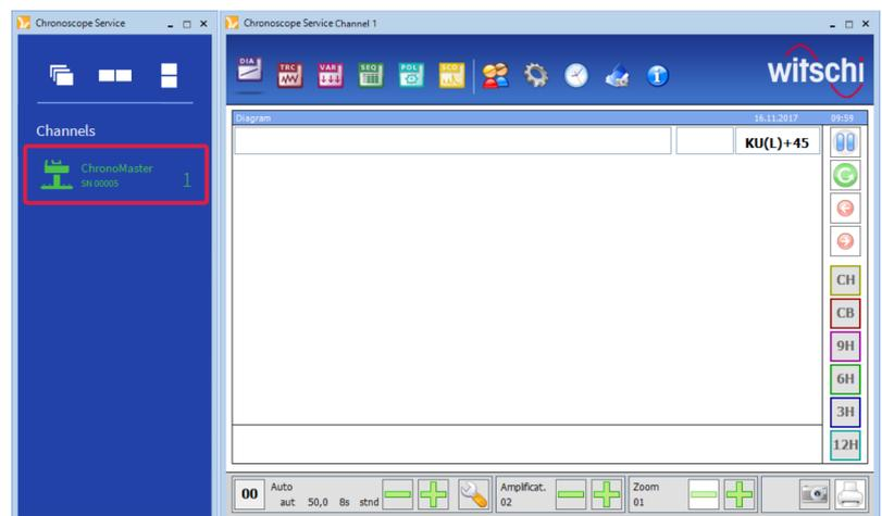
Fig. 7: ChronoMaster identified by the display software
